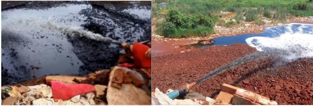
Figure 10. Sludge being washed-down with high-pressure wastewater
